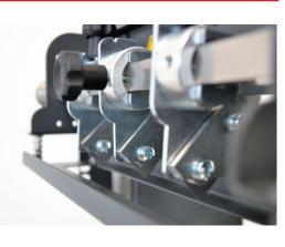
The ultrasonic sensor is used to adjust automatically and electronically the tension on the media despite the roll diameter variation. With this feature it is possible to get extremely tight finished rolls.
