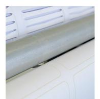
facilitate the matrix removal from the die-cut roll, reducing the risk of tearing and ensuring more precise operation of the machine.
