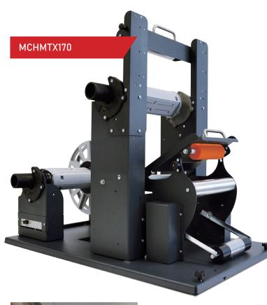
Designed to be installed and work in-line to OKI Pro Series Label Printer, the Matrix Remover is an all-in-one system capable of removing the waste material from the pre die-cut media and rewinding on a 3" cardboard core with the finished printed labels face out
